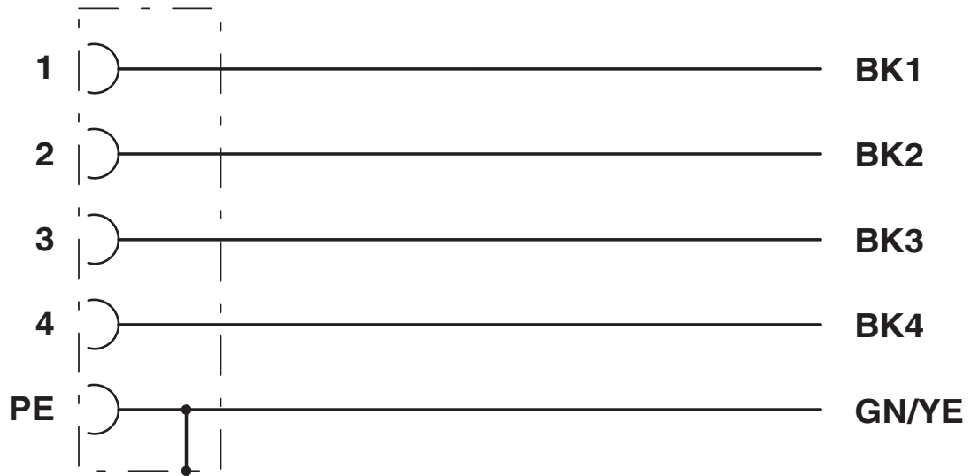
Contact assignment of the M12 socket
