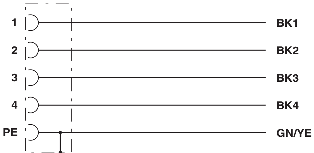
Contact assignment of the M12 socket
