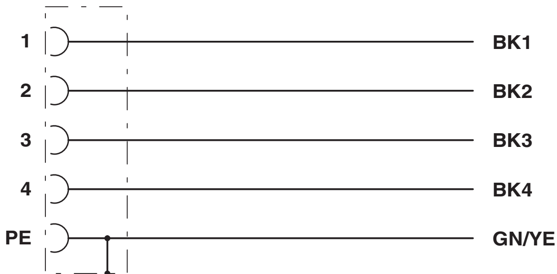
Contact assignment of the M12 socket
