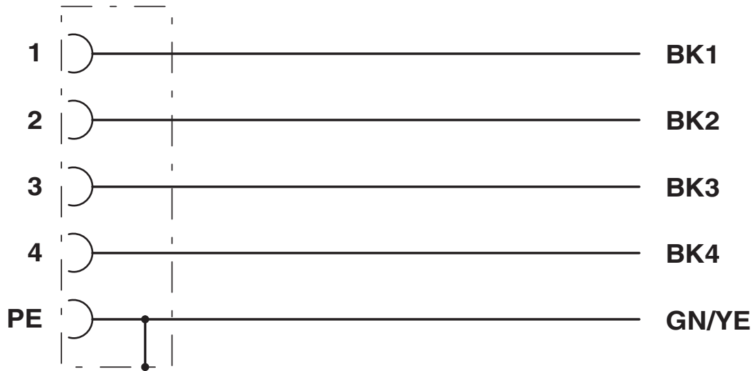
Contact assignment of the M12 socket
