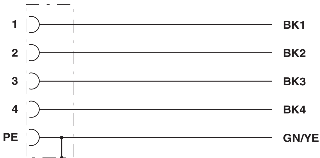
Contact assignment of the M12 socket
