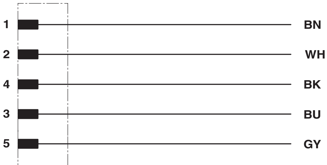
Contact assignment of the M12 connector
