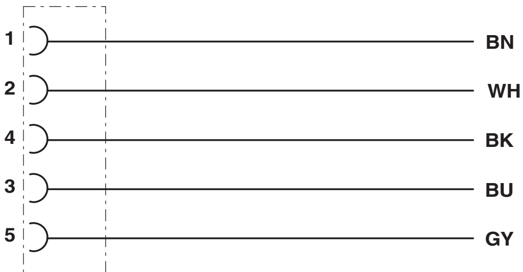
Contact assignment of the M12 socket
