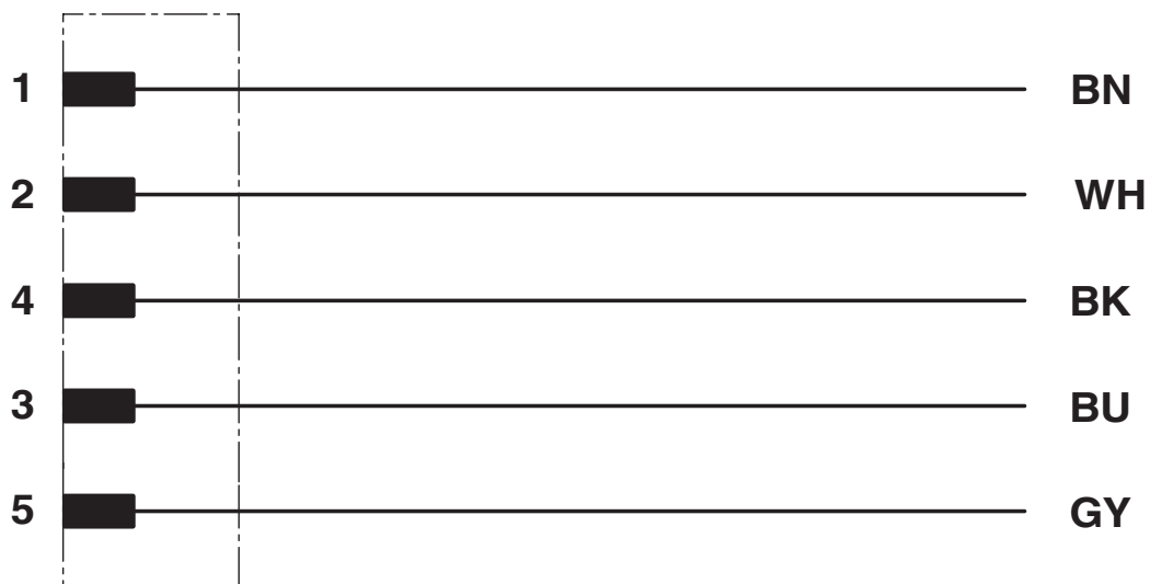
Contact assignment of the M12 plug
