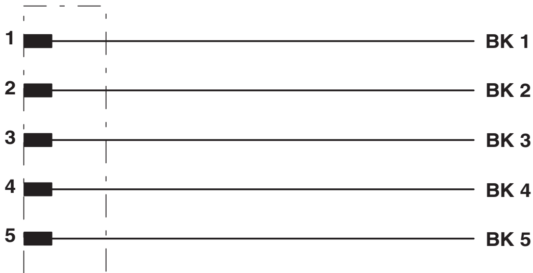
Contact assignment of the M12 socket
