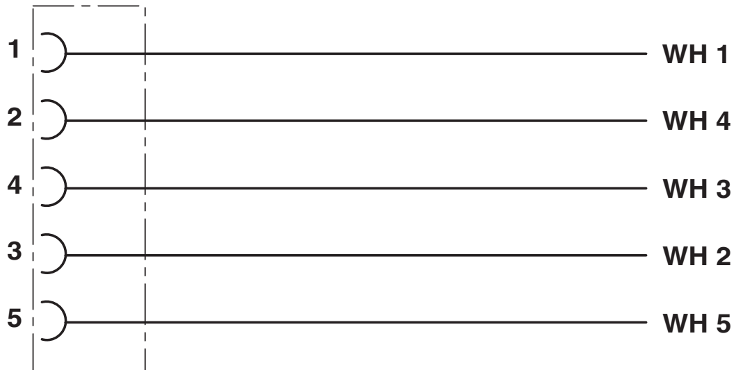
Contact assignment of the M12 socket
