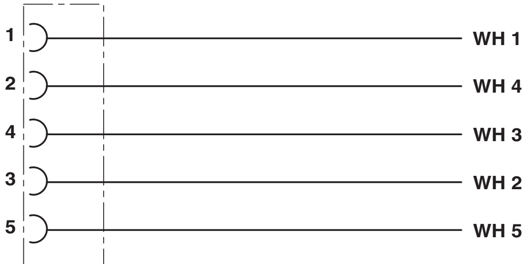
Contact assignment of the M12 socket
