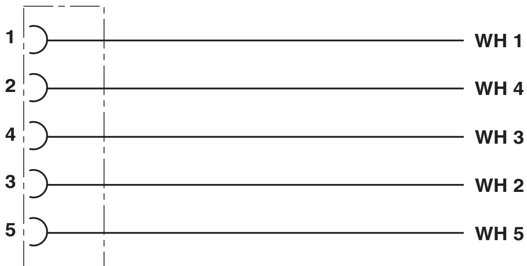
Contact assignment of the M12 socket
