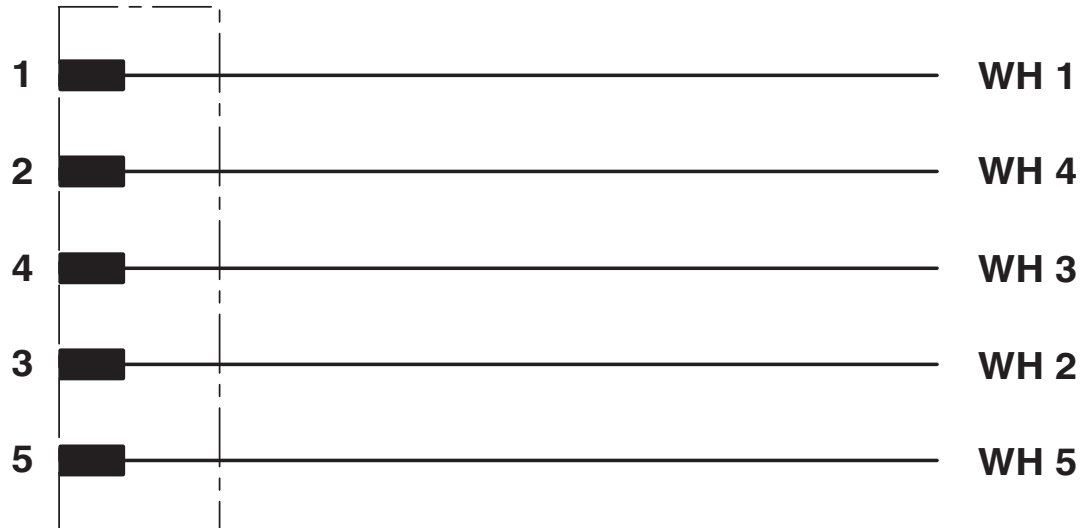
Contact assignment of the M12 plug
