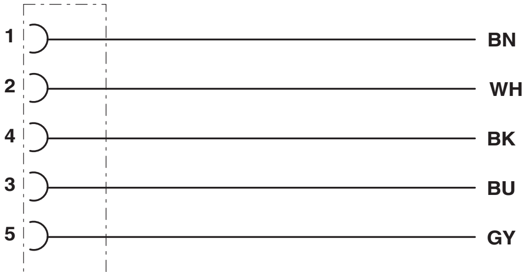
Contact assignment of the M12 socket
