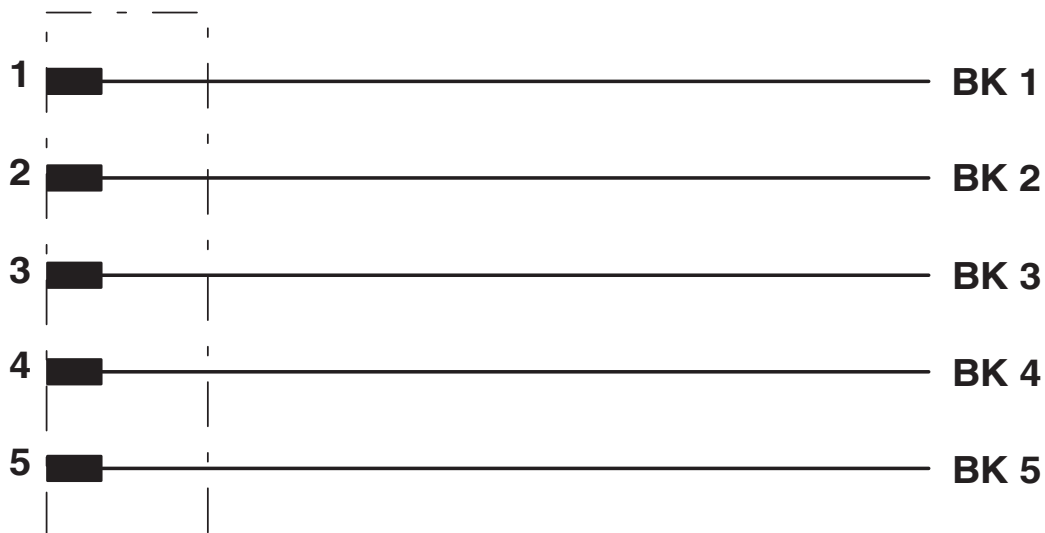
Contact assignment of the M12 socket
