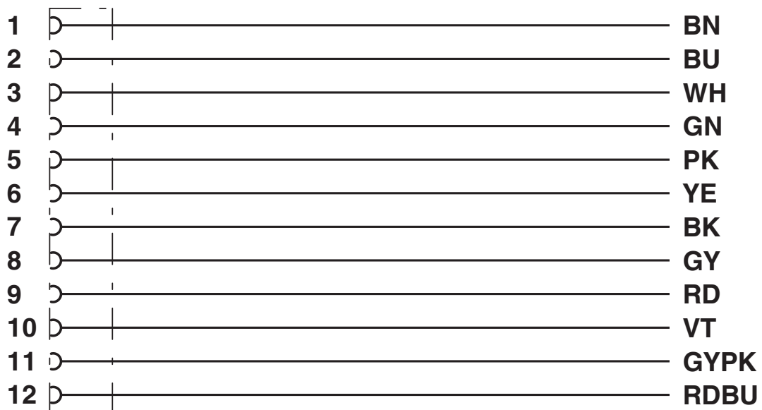
Contact assignment of the M12 socket
