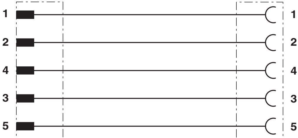
Contact assignment of M8 plugs/sockets
