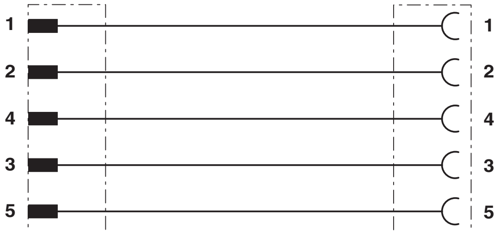
Contact assignment of M8 plugs/sockets
