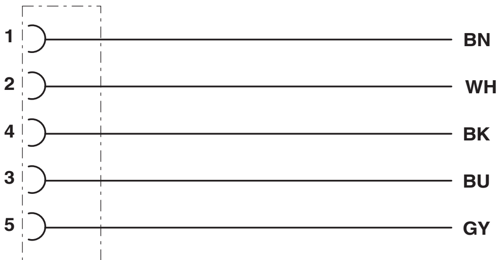
Contact assignment of M8 socket
