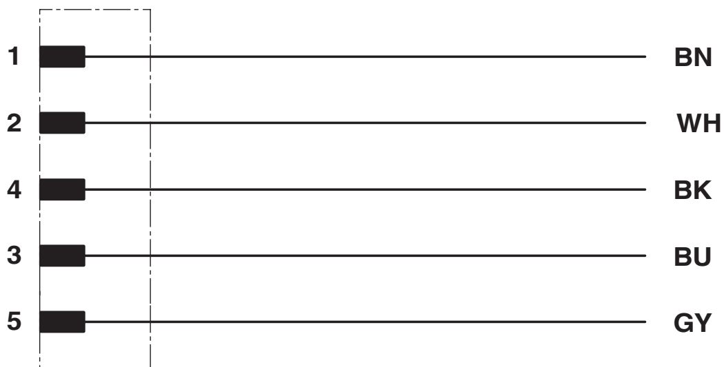
Contact assignment of the M8 plug
