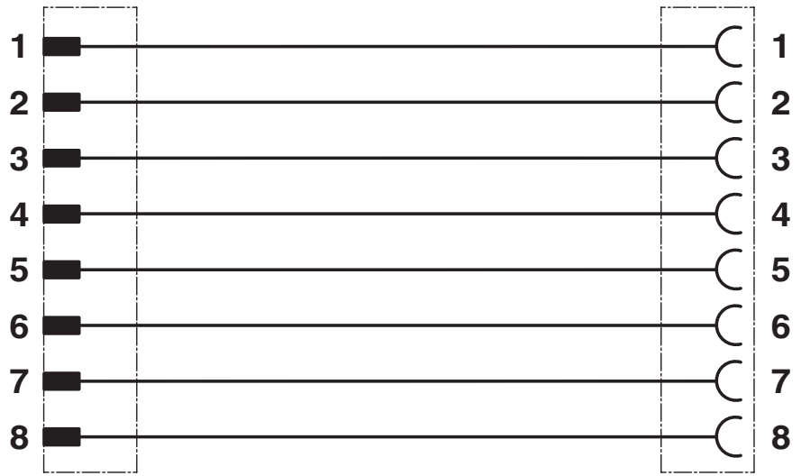
Contact assignment of M8 plugs/sockets
