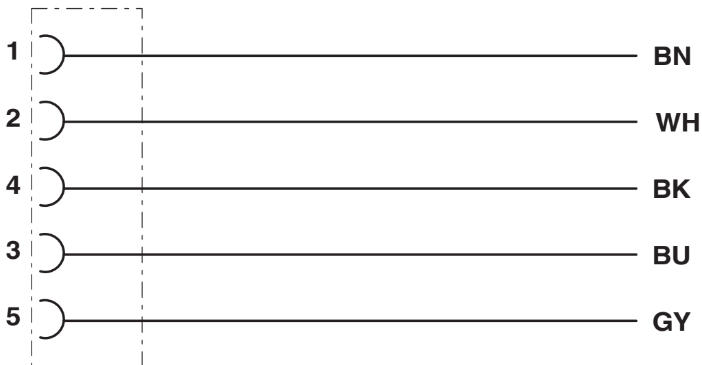
Contact assignment of the M12 socket
