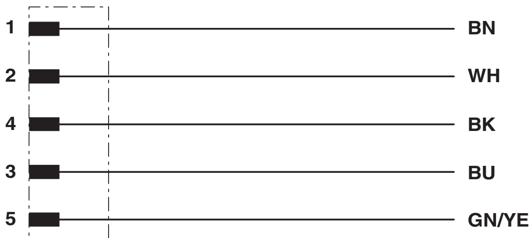
Contact assignment of the M12 plug
