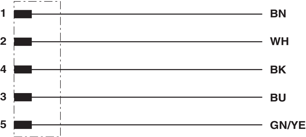
Contact assignment of the M12 plug
