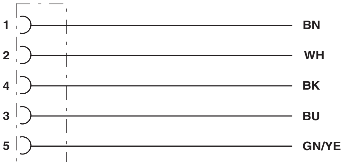
Contact assignment of the M12 socket
