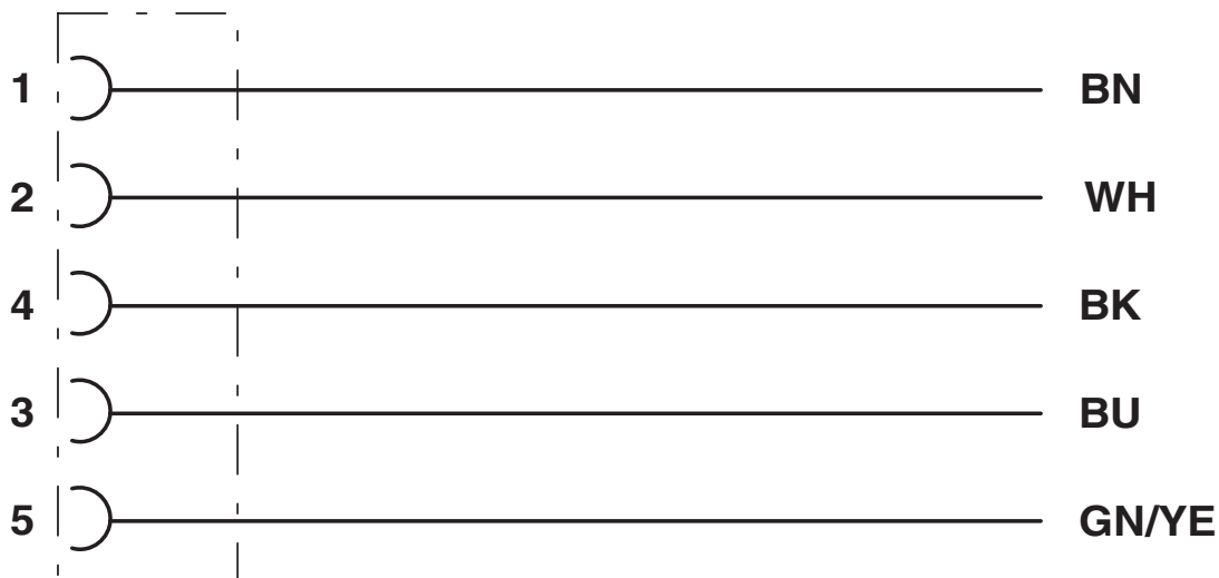
Contact assignment of the M12 socket
