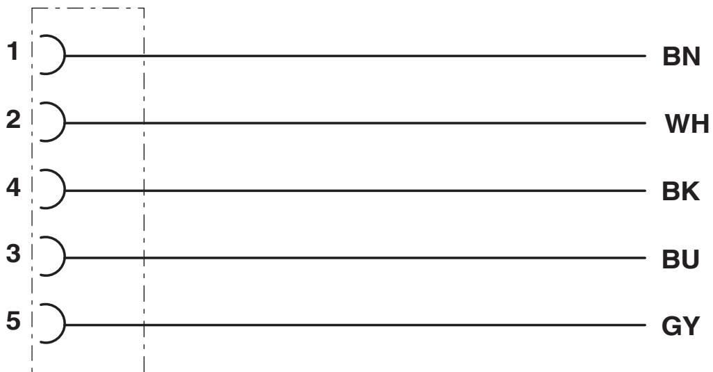
Contact assignment of the M12 socket
