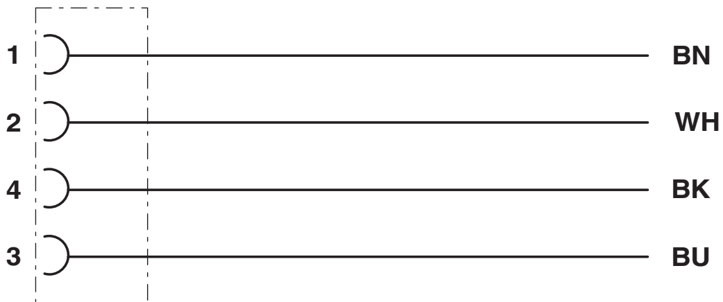
Contact assignment of the M12 socket
