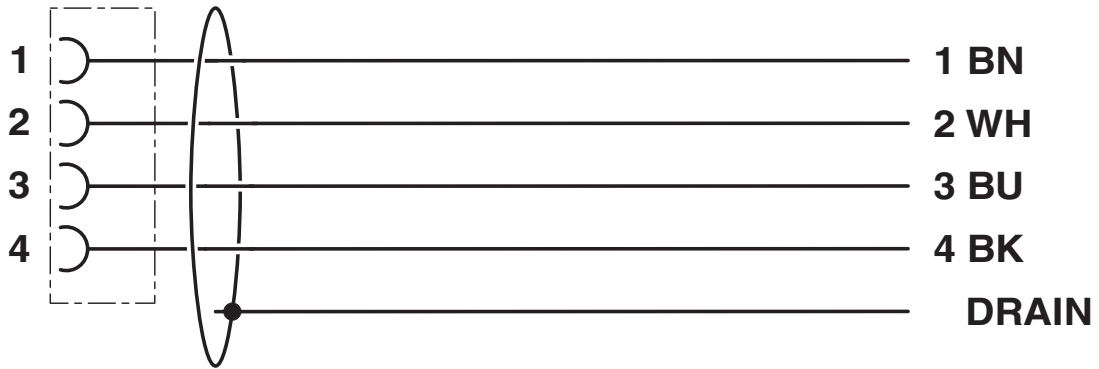
Contact assignment of M8 plugs/sockets
