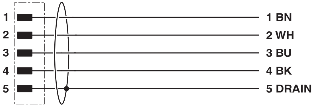
Contact assignment of the M12 plug and the M12 socket
