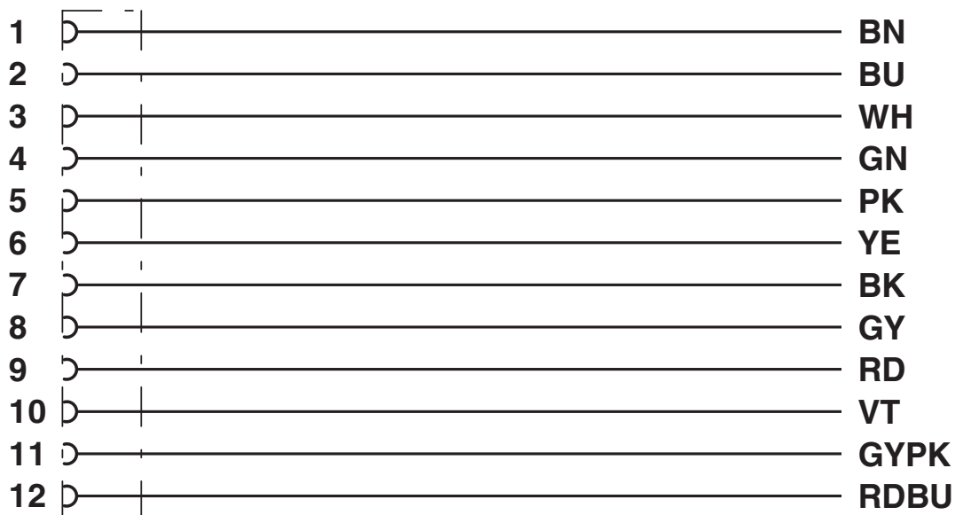
Contact assignment of the M12 socket
