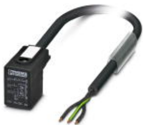
Sensor/actuator cable, 3-position, PUR halogen-free, black-gray RAL 7021, free cable end, on Valve connector BI (11 mm), with 1 LED, connected with Z diode, cable length: 5 m
