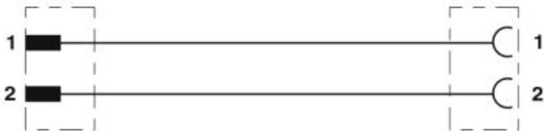
Contact assignment of the super seal plug to the super seal socket
