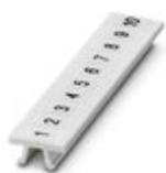
Zack marker strip, Strip, white, labeled, printed horizontally: consecutive numbers 1 ... 10, 11 ... 20, etc. up to 91 ... 100, mounting type: snap into tall marker groove, for terminal block width: 5.08 mm, lettering field size: 4.98 x 10.5 mm, Number of individual labels: 10
