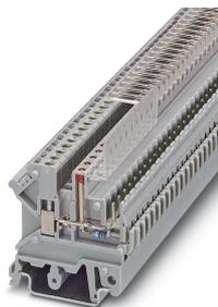
Feed-through terminal block, nom. voltage: 250 V, nominal current: 12 A, connection method: Screw connection, number of connections: 2, number of positions: 1, cross section: 0.2 mm<sup>2</sup> - 4 mm<sup>2</sup>, AWG: 24 - 12, width: 5.1 mm, color: gray, mounting type: NS 32, NS 35/15, NS 35/7,5
