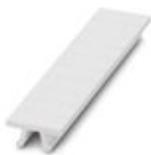
Zack marker strip, can be ordered: Strip, white, labeled according to customer specifications, mounting type: snap into tall marker groove, for terminal block width: 5.08 mm, lettering field size: 4.98 x 10.5 mm, Number of individual labels: 10
