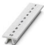
Zack marker strip, Strip, white, labeled, Printed vertically: consecutive numbers 1 ... 10, 11 ... 20, etc. up to 91 ... 100, mounting type: snap into tall marker groove, for terminal block width: 5.08 mm, lettering field size: 10.5 x 5.15 mm, Number of individual labels: 10
