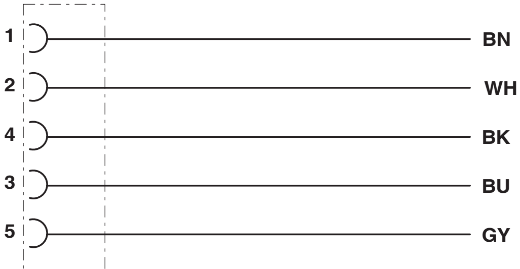
Contact assignment of the M12 socket
