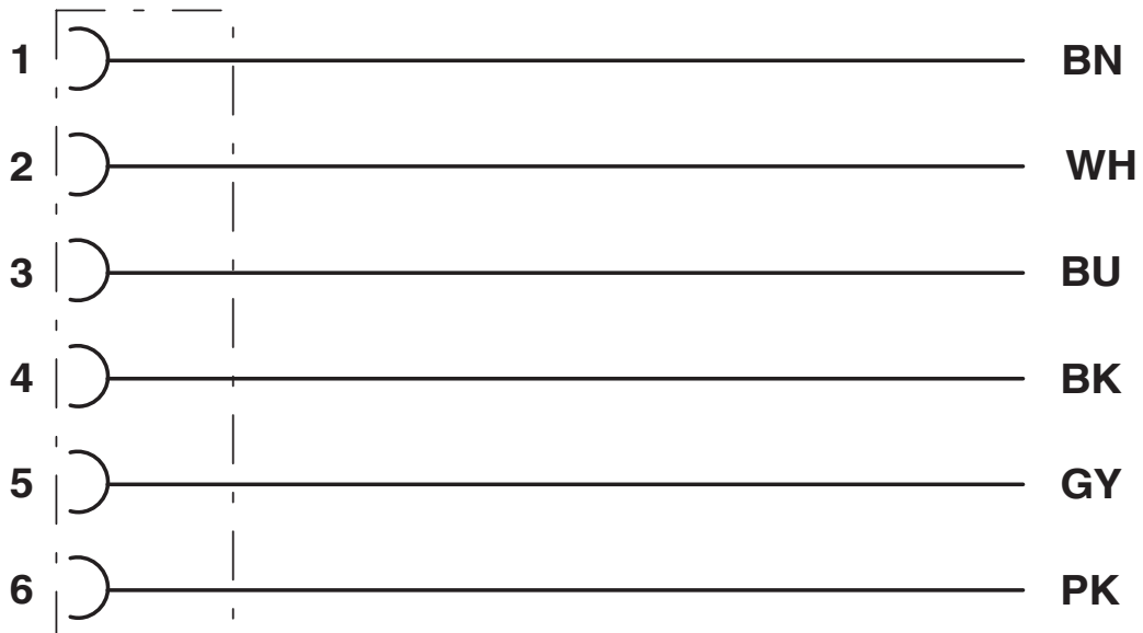
Contact assignment of M8 socket
