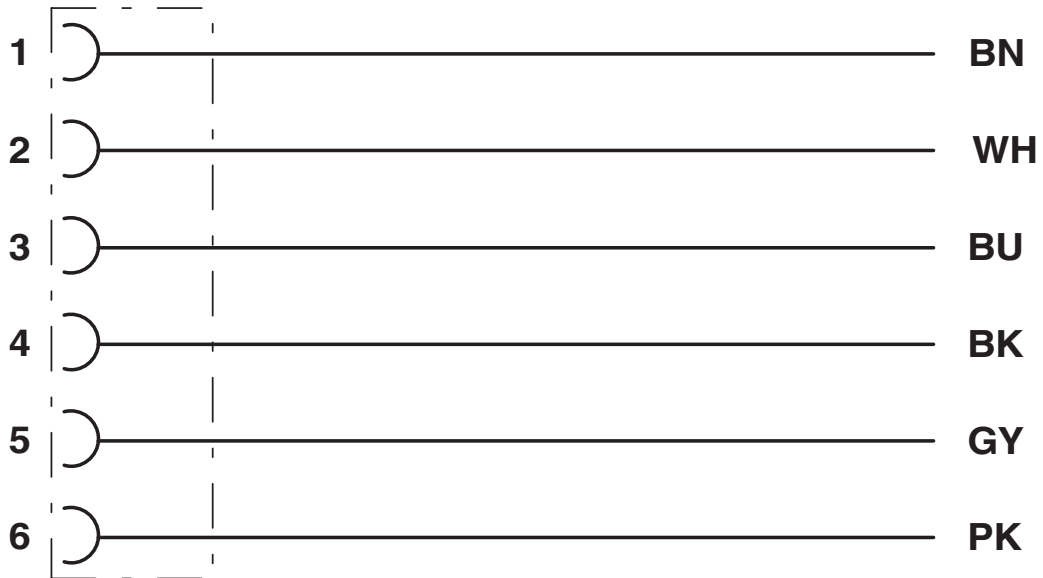
Contact assignment of M8 socket
