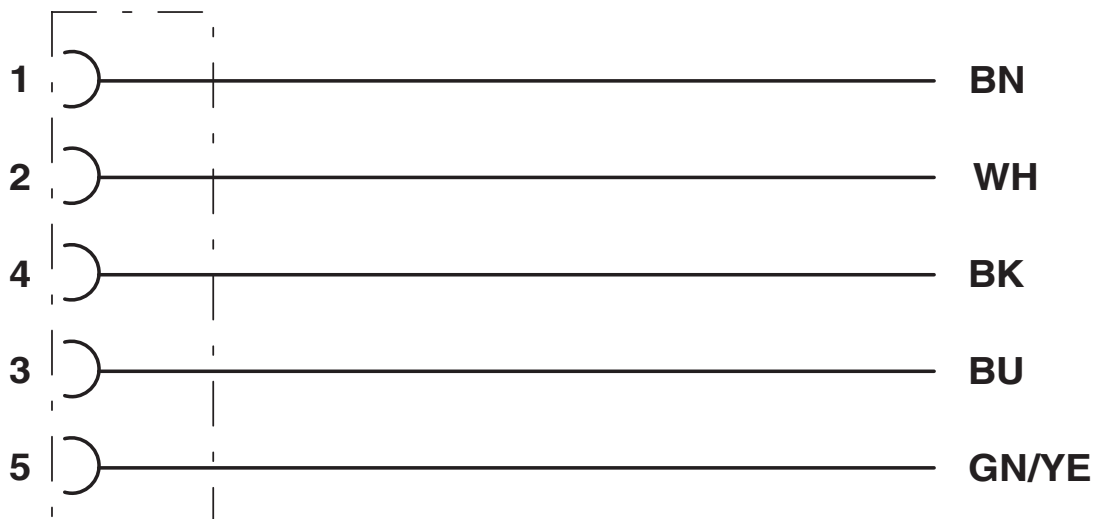
Contact assignment of the M12 sockets
