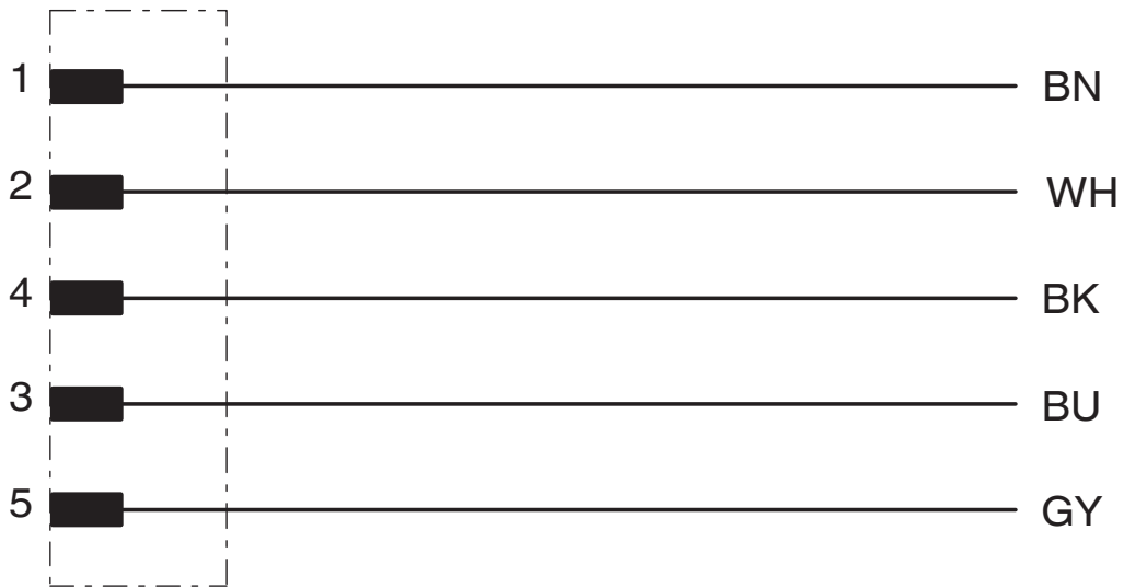
Contact assignment of the M12 plug
