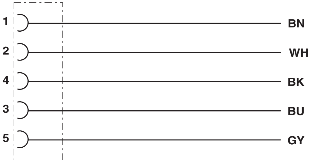
Contact assignment of the M12 sockets
