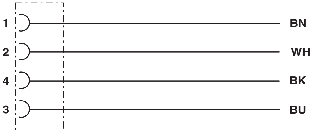
Contact assignment of the M12 socket
