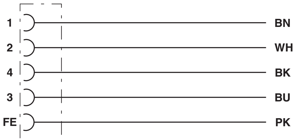
Contact assignment of the M12 socket
