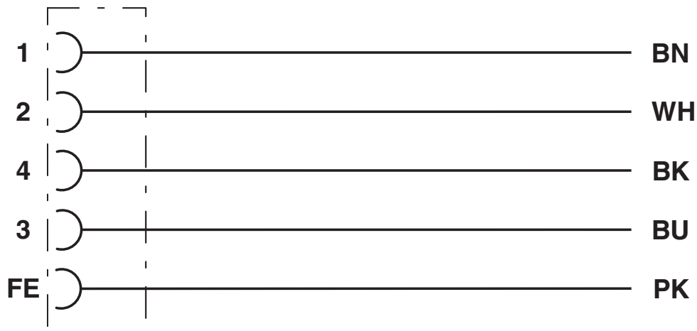
Contact assignment of the M12 socket
