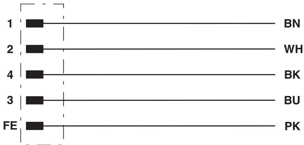
Contact assignment of the M12 plug
