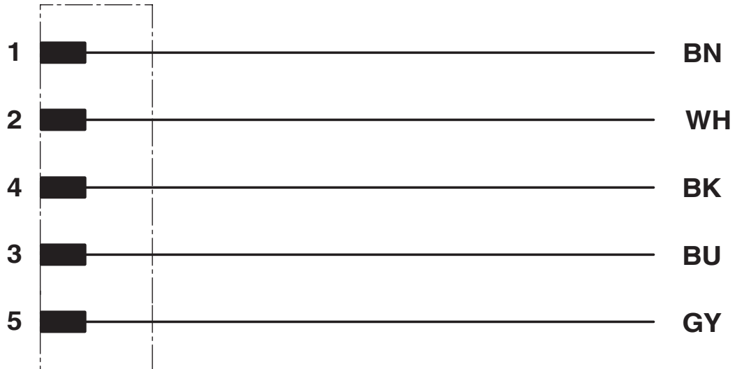
Contact assignment of the M12 plug
