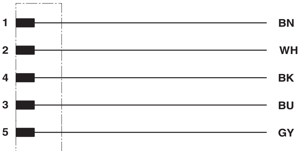
Contact assignment of the M12 plug
