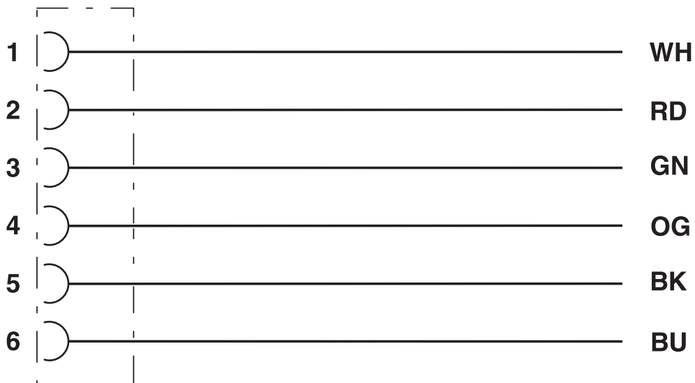
Contact assignment of 7/8" socket
