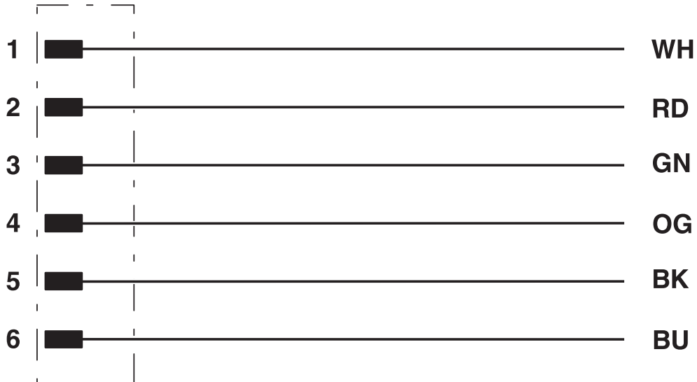
Contact assignment of 7/8" plug
