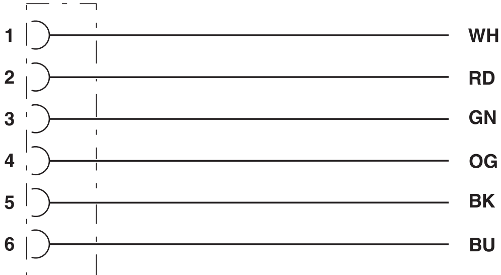
Contact assignment of 7/8" socket
