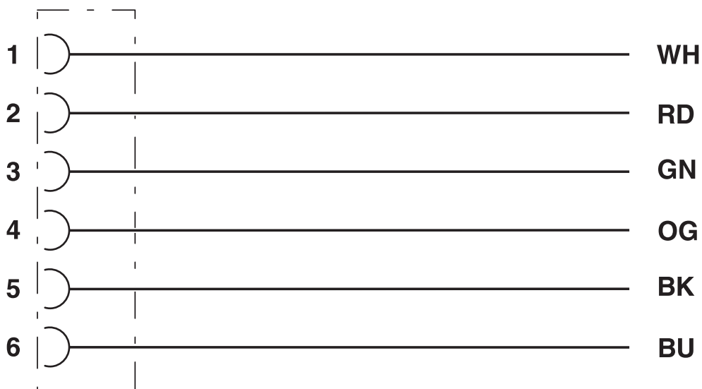
Contact assignment of 7/8" socket
