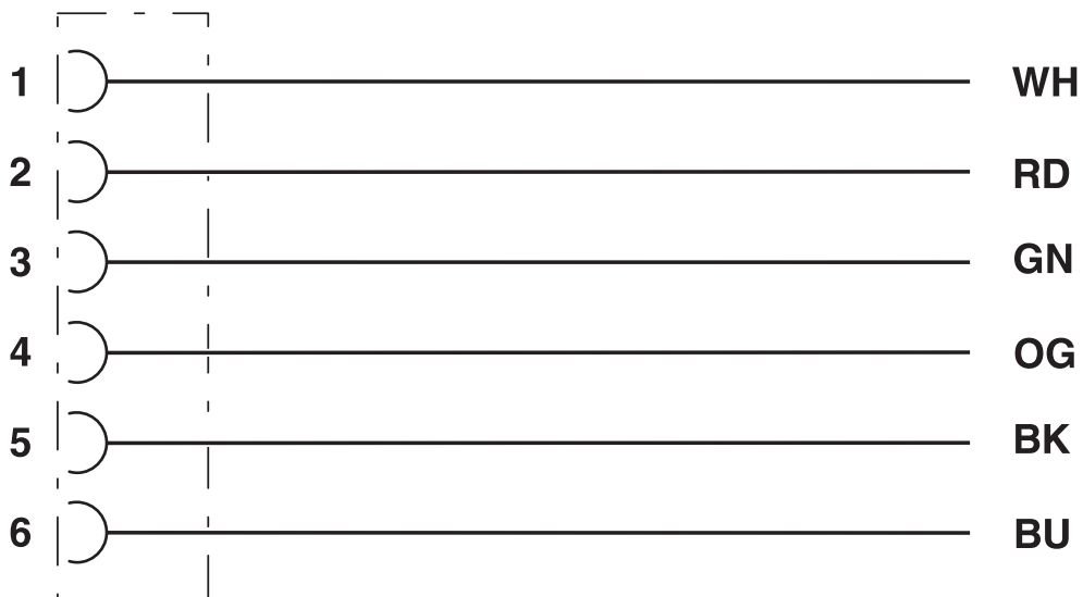
Contact assignment of 7/8" socket
