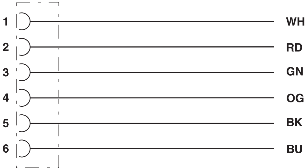
Contact assignment of 7/8" socket
