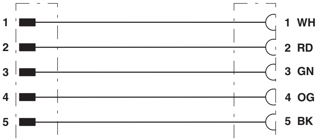
Contact assignment of 7/8" plugs/sockets
