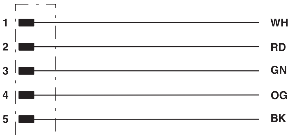
Contact assignment of 7/8" plug
