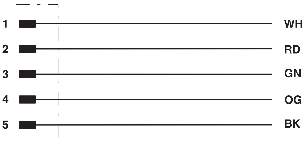
Contact assignment of 7/8" plug
