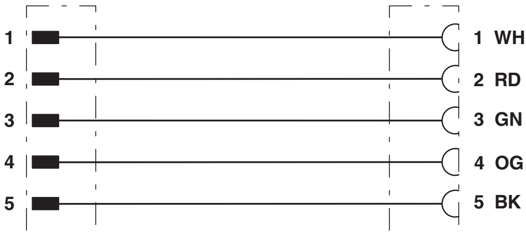
Contact assignment of 7/8" plug
